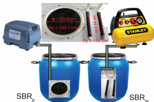
Fig. 1. The laboratory test stand for testing wastewater treatment efficiency in SBR p and SBR m
